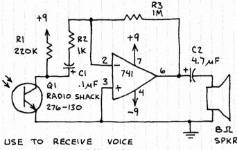
MODULATED LIGHT WAVES. OK TO USE SINGLE POLARITY POWER SUPPLY FOR NON-VOICE RECEPTION.
